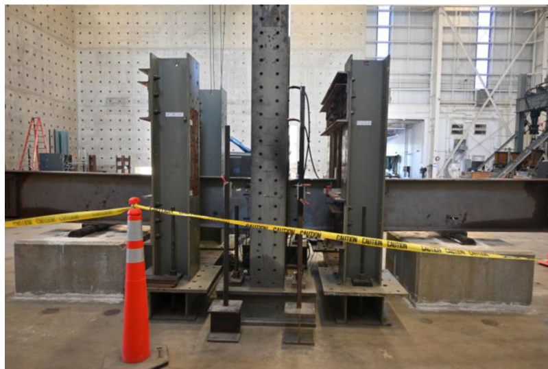
Figure 5.25 Specimen 7 flexural yielding.
