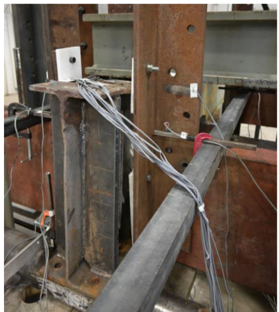
Figure 5.11 Specimen 3 web condition at the support.
