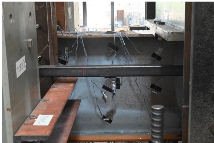
Figure 3.18 Specimen 6 after inducing the section loss.
