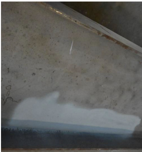
Figure 3.20 Specimen 7 after inducing the section loss.
