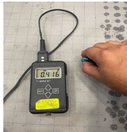
Figure 3.1 Section loss measurements using an ultrasonic thickness gauge.
