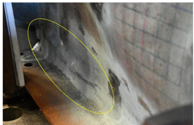
Figure 5.21 Specimen 6 OOP web displacement at the bottom (SP14).
