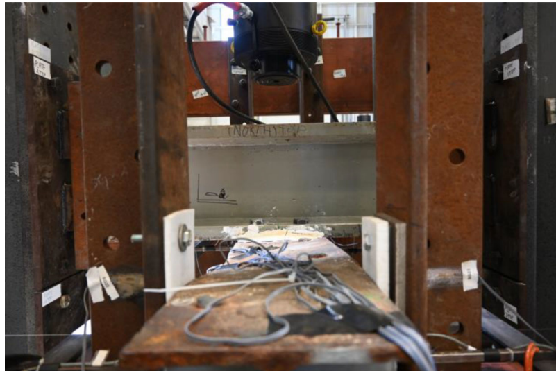
Figure 5.23 Tilting of top flange and spreader beam.
