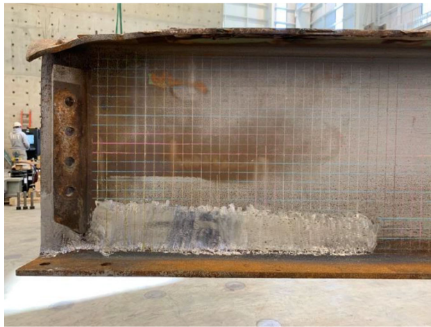
Figure 3.14 Specimen 4 after inducing section loss artificially through grinding.
