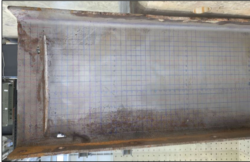
Figure 3.7 Specimen 3 and grids on the web where the remaining thickness is measured.
