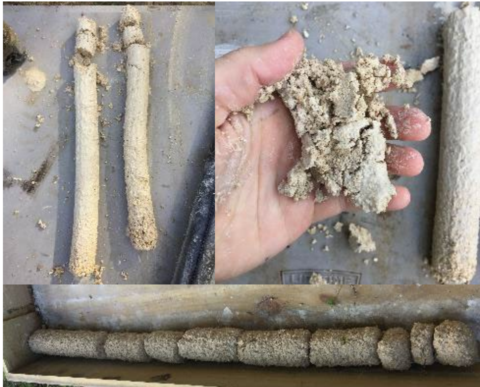
Figure 4-17. Synthetic limestone representing extremely weathered Florida limestone.
