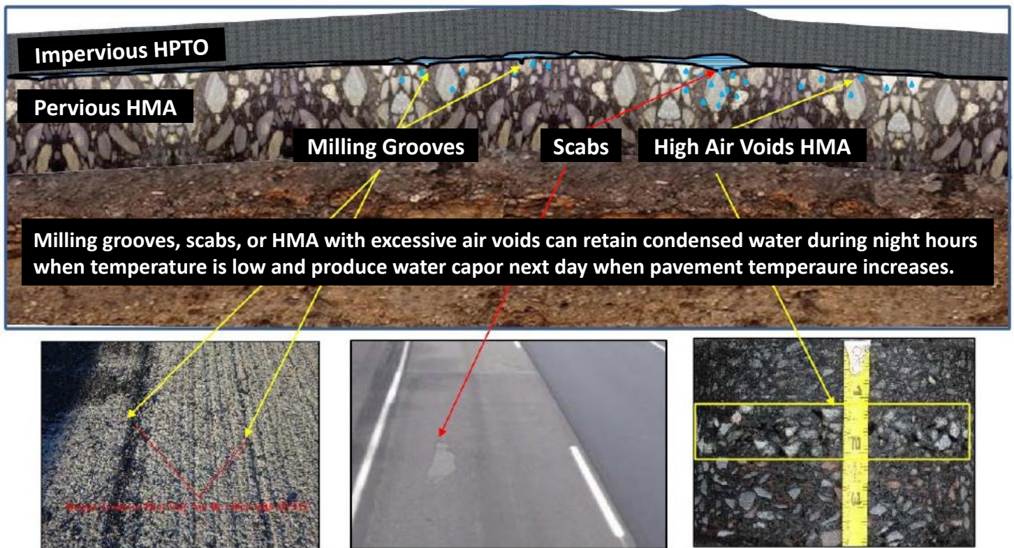
Figure 10. HPTO blistering. Source: NJDOT
