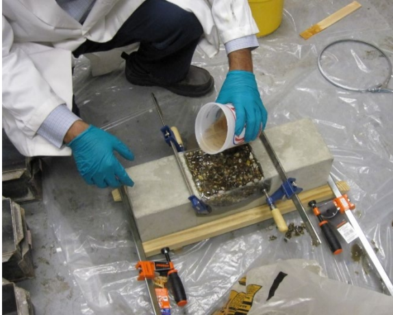
(a) Application of epoxy over aggregate
