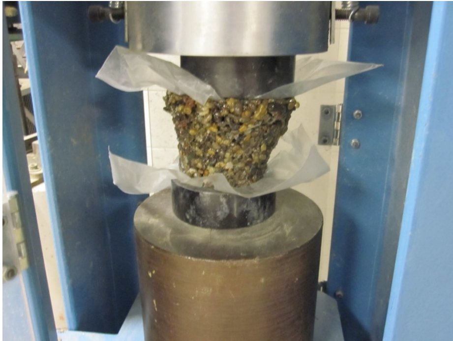
Figure 2.13 Epoxy Mortar Compressive Strength Test at 3 Hours After Placing the Mortar in Cylinder Molds
