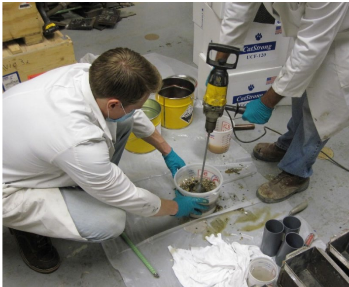
Figure 2.5 Preparation of Sikadur 52 epoxy mortar mix
