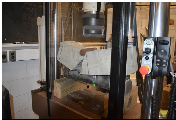
(a) Failure of control beam (P1-B1)
