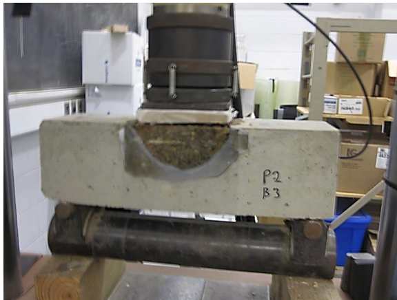
(a) Dynamic loading of Beam 3 (P2-B3)
