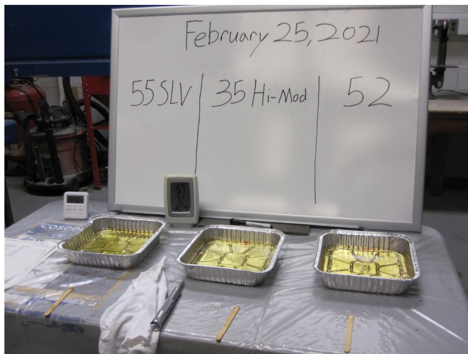
Figure 2.8 Specimens for Epoxy Set-Time Tests
