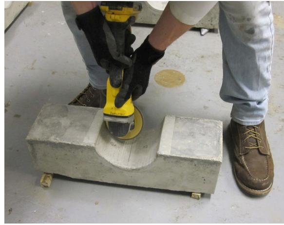
(b) Roughening bond surface (only P1-B6)
