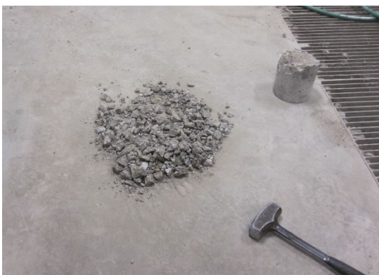
(a) Concrete from cylinder tests crushed for use in patch repair
