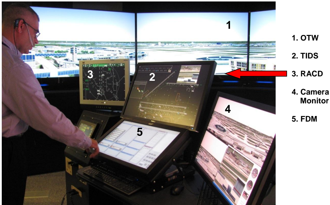
Figure 4. Display configuration for the SNT HITL 2 simulation included the (1) Out-the-Window view, (2) Tower Information Display System, (3) Remote ARTS Color Display, (4) Camera Monitor, and (5) Flight Data Manager.
