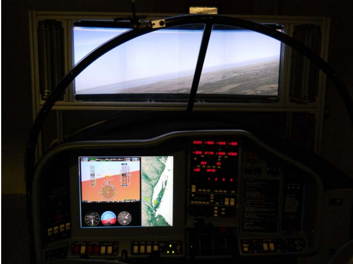
Figure 3. Micro-Jet cockpit simulator.
