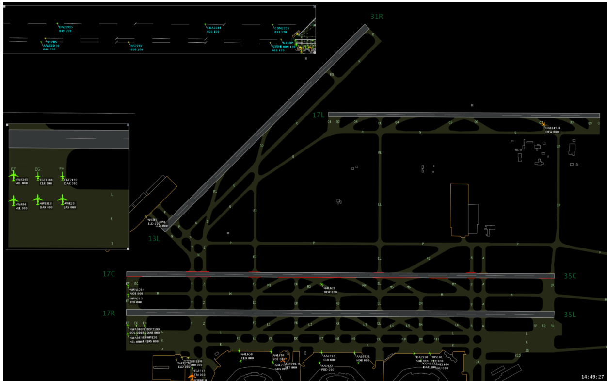
Figure 1. An example of the Tower Information Display System.
