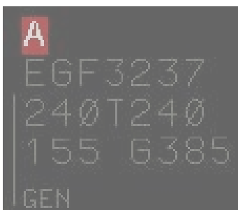
Figure 5. Example of conflict probe notification in the data block in the flashing/urgent condition.
