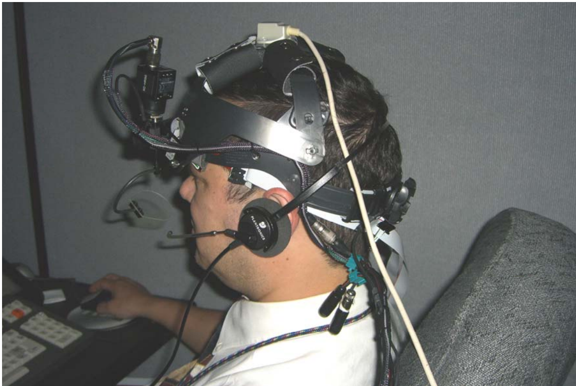
Figure 10. The picture shows eye movement tracking and fNIR patch partly hidden under the eye movement tracking system.
