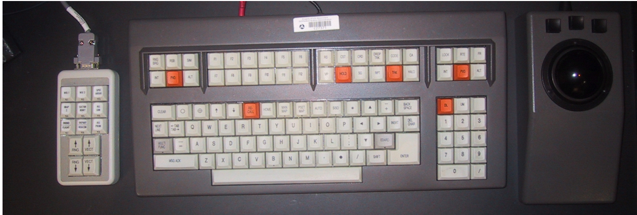
Figure 4. Data entry devices available on the controller desk area.
