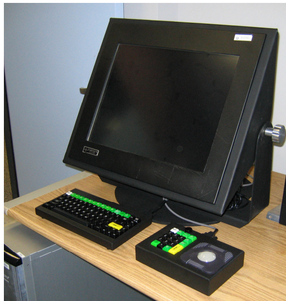
Figure 5. An EFDI controller workstation including touch sensitive display, display mount, ASDE-X keyboard, and trackball/keypad.
