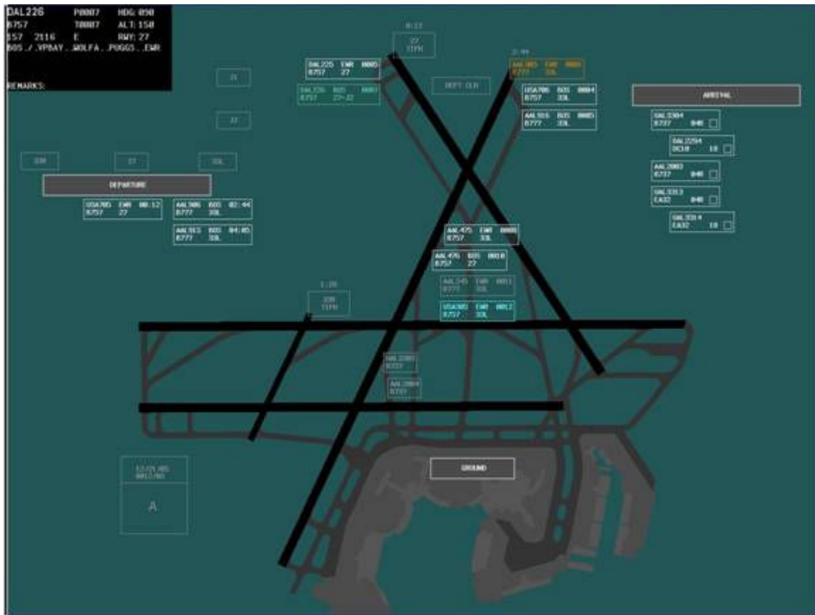
Figure 3. The primary elements of the P-S EFDI including flight data elements, readout area, buttons, and system information window.
