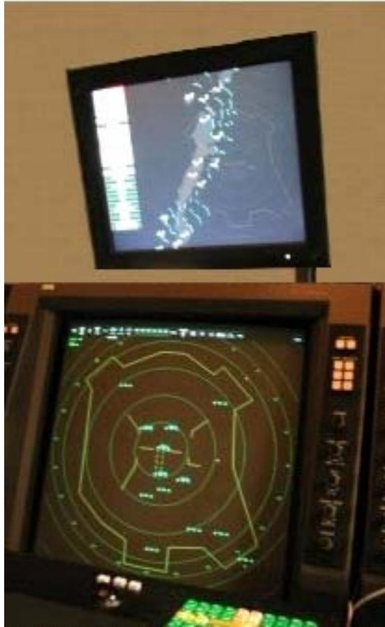
Figure 3. The WIDS and TCW configuration used during the simulation (WIDS top display, TCW bottom display).
