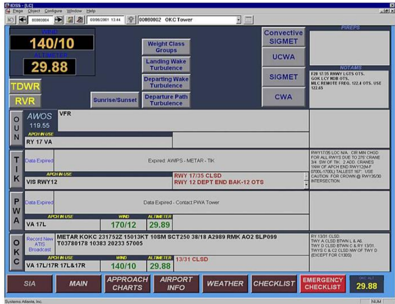
Figure 10. An illustration of how the color red may be used to indicate emergency conditions.
