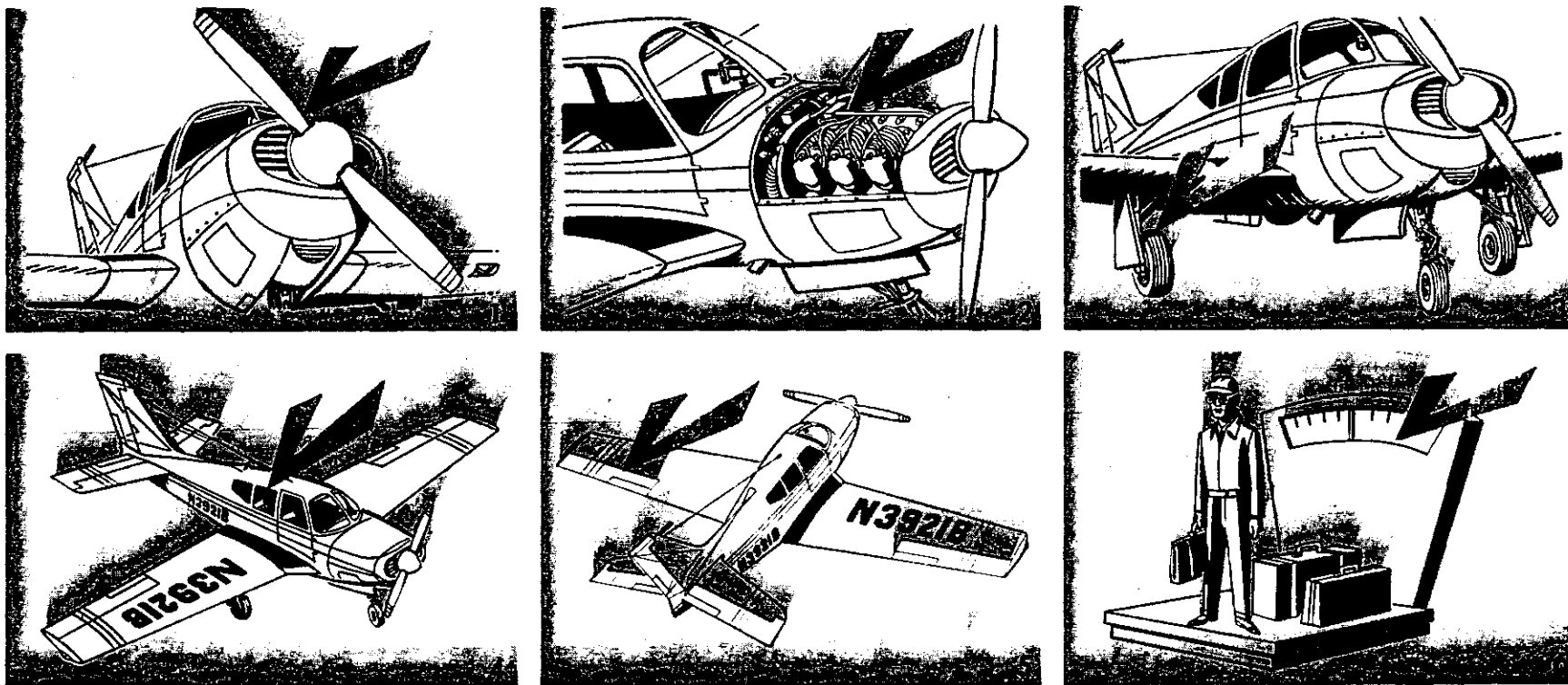
Figure 88. Preflight inspection should include at least: (1) propeller; (2) engine; (3) landing gear; (4) wings and fuselage; (5) control surfaces and controls; (6) weight of baggage and passengers.
