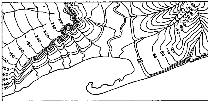
Figure 64. Altitude, form, and slope of terrain as indicated by contour lines and numerals (U.S. Geological Survey).
