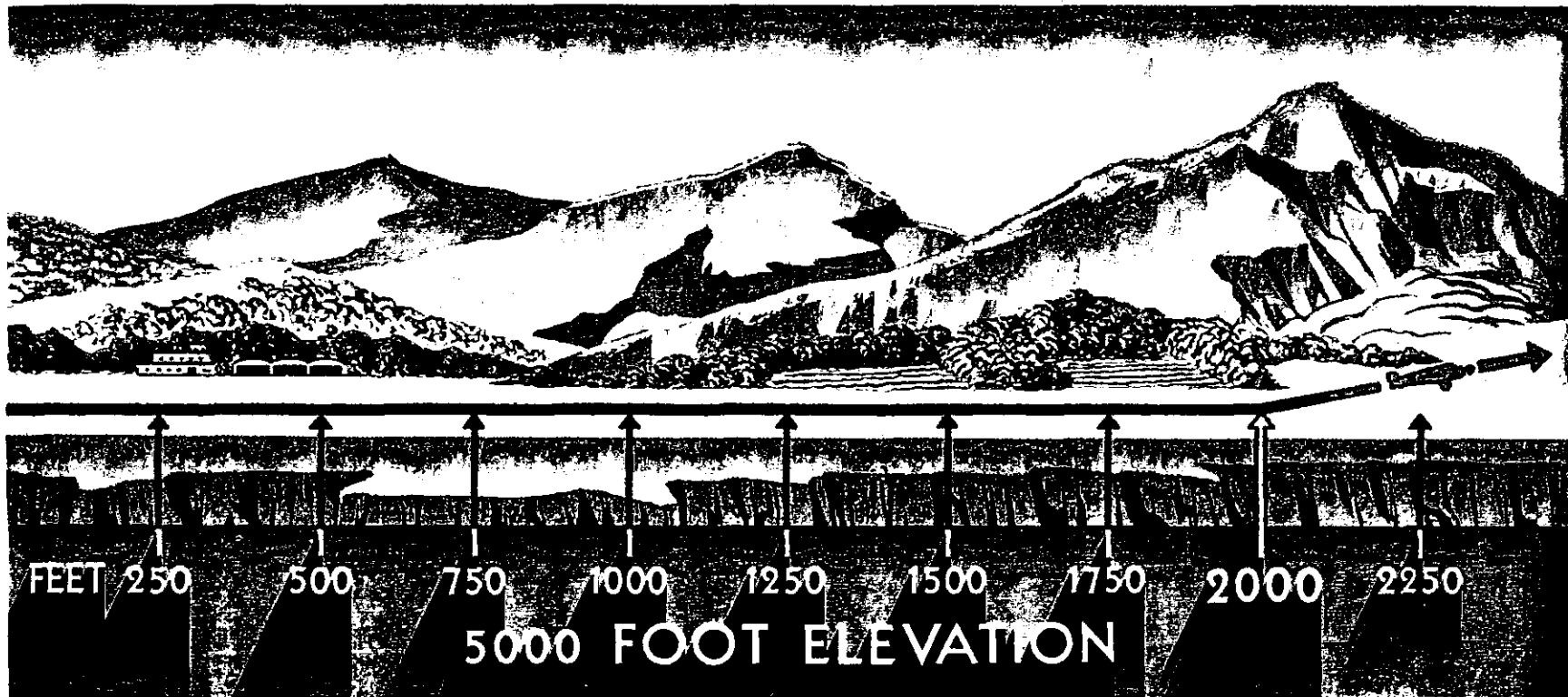
Figure 27. The distance required for takeoff increases with the altitude of the field.
