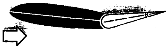
Up position of the elevators is required to hold the nose in the level flight attitude
