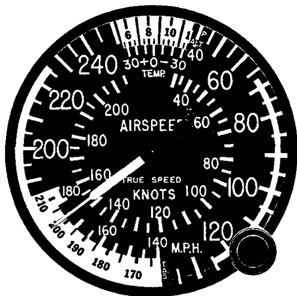
Figure 3-5. Airspeed indicator showing color-coded marking system.
