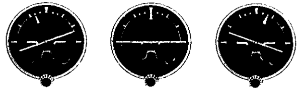
FIGURE 19. Artificial horizon (attitude indicator) indications.
