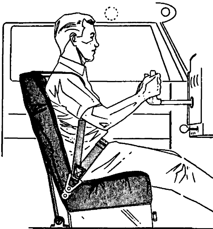
FIGURE 9.8.—Floor mounted inertia reel—double over-the-shoulder type harness.
