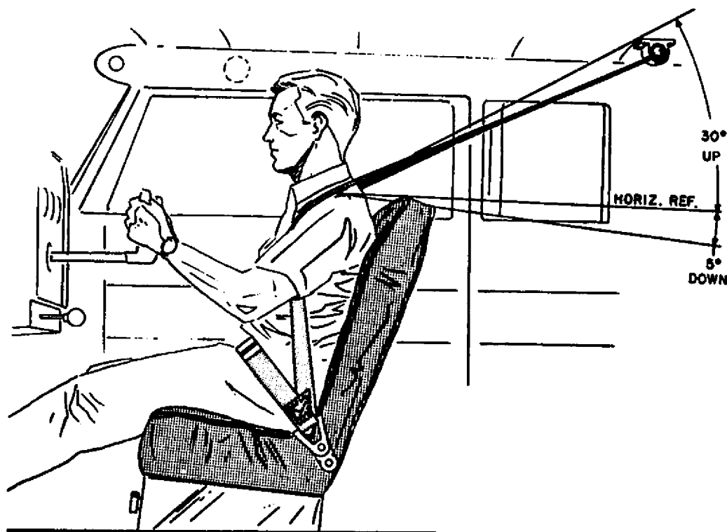
FIGURE 9.6.—Ceiling mounted inertia reel—double over-the-shoulder type harness.
