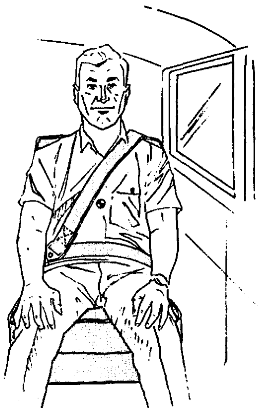
FIGURE 9.17.—Correct Installation—Single Diagonal Type Harness.
