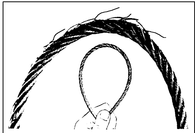
FIGURE 7-16. Cable inspection technique.
