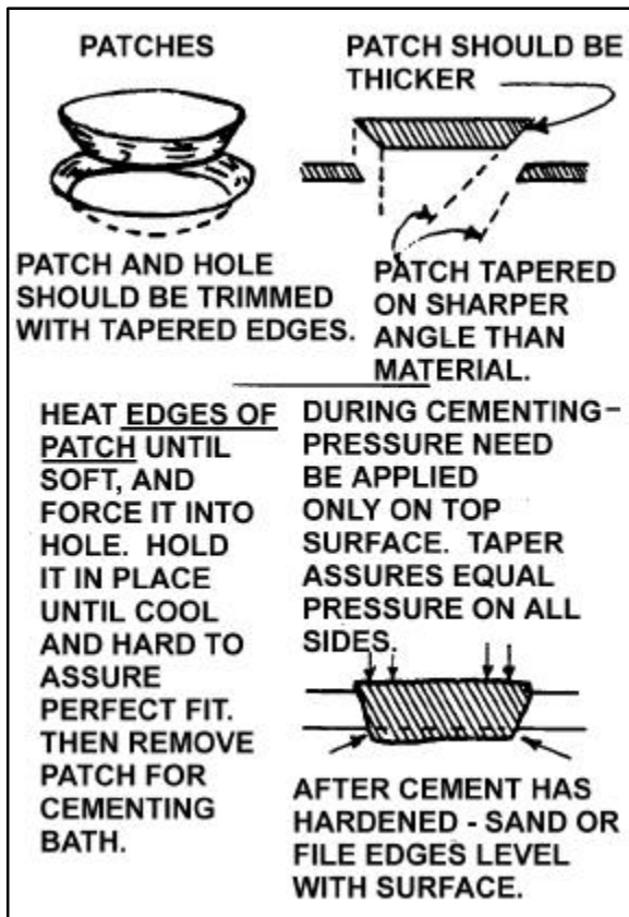
FIGURE 3-23. Plug patch repair.
