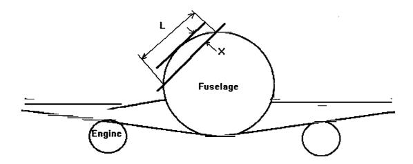
Typical, but not the only tangential projection possible. L can be assumed to be the sector distance (i.e., straight line). X is the engine fragment dimension obtained from AC 20-128A.
