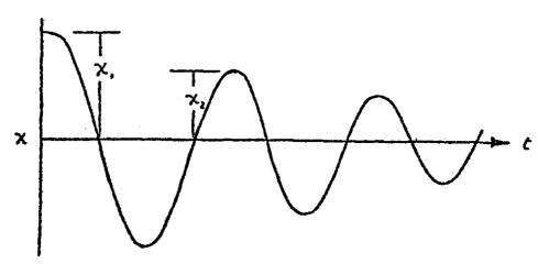
The log decrement,  $\int$ , is then equal to  $\ln(\frac{x_1}{x_2})$ ; or as  $\frac{0.693}{n}$  where n = no. of cycles to 1/2 amplitude; i.e.:  $\frac{x_1}{x_2} = 2$ .
