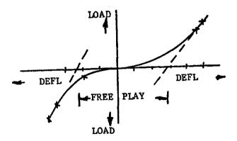
Free play is then defined by extending the best straight lines thru zero. System stiffness may then be obtained from the slopes of the curves away from the zero point.
