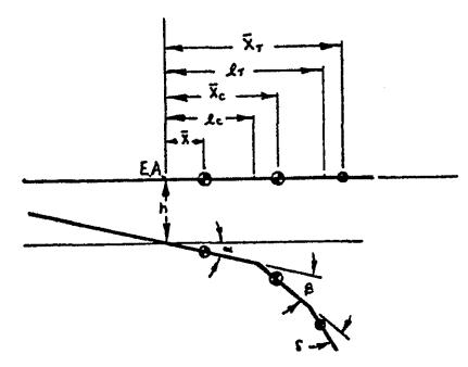
The equation of Motion is:  $\left[ \overline{M} \right] \left\{ \overline{q} \right\} + (1 + i \cdot g) \left[ \overline{K} \right] \left\{ \overline{q} \right\} = \left\{ \overline{E}_A \right\}$
