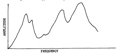
Although duplication of peak responses will result, it is advantageous to obtain frequency response records with a reference pickup positioned on each of the main surfaces and fuselage at a specific shaker location. This will reduce the chances of overlooking modes.
