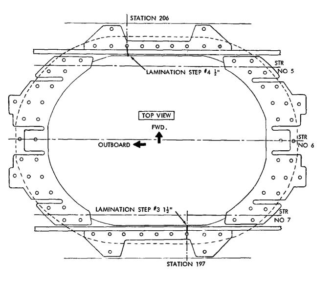
FIGURE 1. CRACKS IN WING FUEL ACCESS DOOR LAND AT WS 197 AND WS 206.
