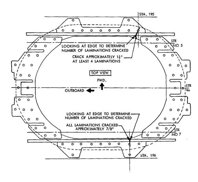
FIGURE 2. CRACKS IN WING FUEL ACCESS DOOR LAND AT WS 195 AND WS 196.
