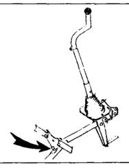
Piper Model PA-38-112 Rudder Assembly, P/N 77611-02 The rudder controls jammed when deflected approximately half travel to the left during flight. A significant amount of pressure had to be applied to the right pedal in order to free the controls. Subsequent ground investigation revealed the leading edge skin of the rudder upper fairing had caught on the top of the vertical stabilizer. The difficulty was experienced at approximately 65 hours aircraft time in service.
