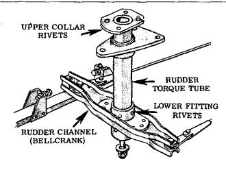
It is suggested that rudder control systems be periodically inspected, particularly after high wind conditions have existed, even if gust locks were installed. It is recommended that walkaround preflight inspections be conducted with a control lock on the rudder pedals and the rudder gust lock removed. If significant rudder movement is apparent when pushed from side to side by hand, the rivets may be sheared, and need for further, more detailed inspection is indicated.
