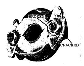
Bendix Magneto Model S-1200 Series Distributor Gear
