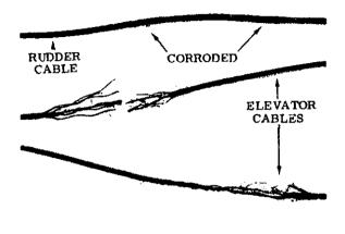
A pilot reported loss of elevator control during takeoff roll. Investigation revealed separation of the elevator control cable and severe corrosion of both the elevator and rudder cables between fuselage stations 353 and 377. The aircraft time in service was 9300 hours. Inspection of another aircraft with 8400 hours time in service disclosed control cable corrosion in the same area, but not as severe.
