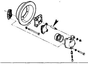
Cessna Control Wheel Model 182, 206, 207 Attach Screws and 210 Series
