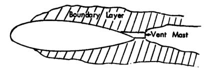
CLASS 2 VENT MAST DISCHARGING INTO FREE STREAM
