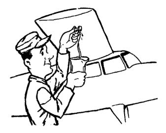
Examine the fuel samples for water and dirt contamination. If present, it will collect at the bottom of the container and should be easily detected. Continue to drain fuel from the contaminated sump until certain the system is clear of all water and dirt.
