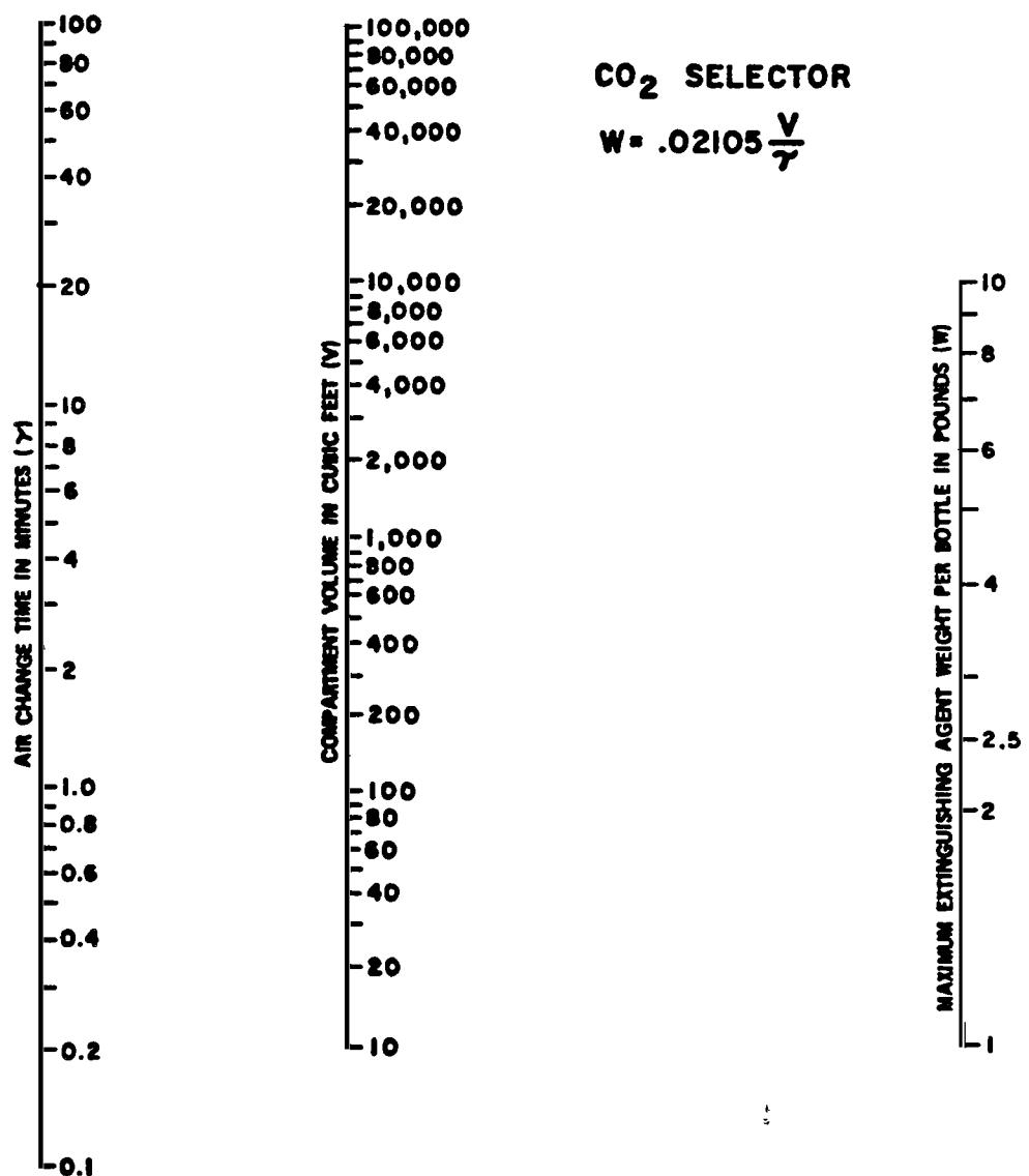
NOTE: Due to the effect of CO<sub>2</sub> on human respiration rate, the allowable CO<sub>2</sub> would be reduced by a factor of six from the amount allowed by the CO<sub>2</sub> nomograph to reduce changes in human respiration rates (Ref. Paragraph 8f(5) of this AC).
