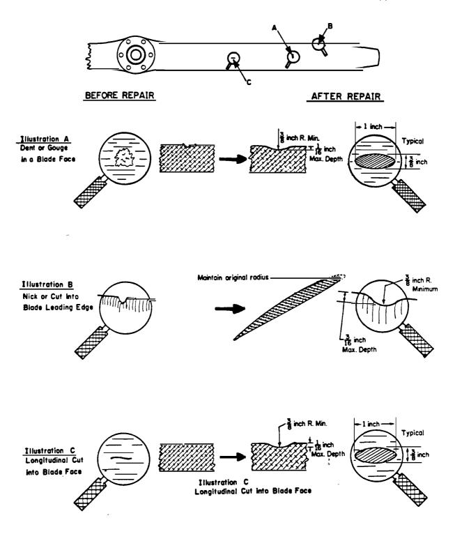
Figure 1. Techniques for Repair of Blade Damage
