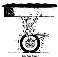
8. REQUIRED MAINTENANCE. During the annual, 100-hour or progressive landing gear inspection cycle, the aircraft is placed on jacks and the gear completely inspected for condition, rigging, and proper operation, including the warning system. Intermediate inspection and servicing will further ensure against landing gear system malfunction.
