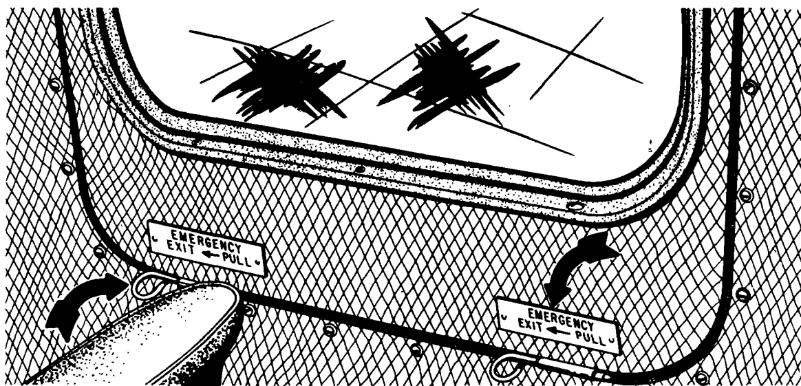
FIGURE 1-14. Emergency exit checkpoints.
