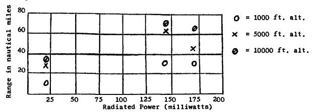
(Altitude of "detector" aircraft shown at 1,000, 5,000, 10,000 feet levels.) The graph shows only the maximum range without reference to aircraft heading, atmospheric conditions, or geographical area. (Note: The graph is intended to show potential range capability vs. power output as related to altitude and has no bearing on the individual manufacturer or his equipment.)
