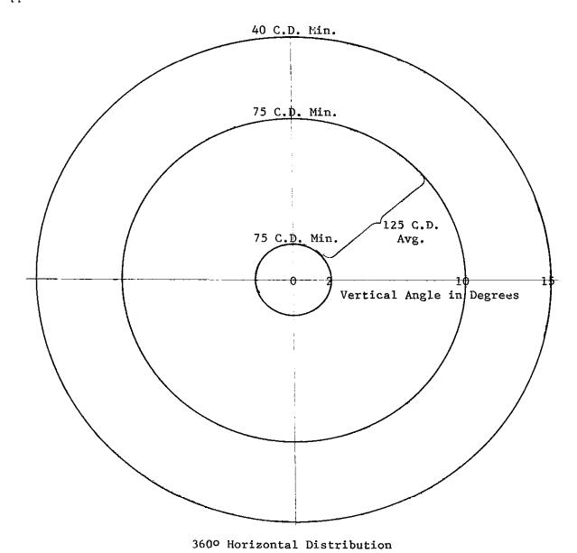
FIGURE 2. Isocandela Curve for Minimum Output in White Light for L-861 Medium Intensity Edge Light.
