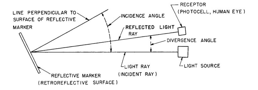
FIGURE I SKETCH ILLUSTRATING THE INCIDENCE AND DIVERGENCE ANGLE OF
