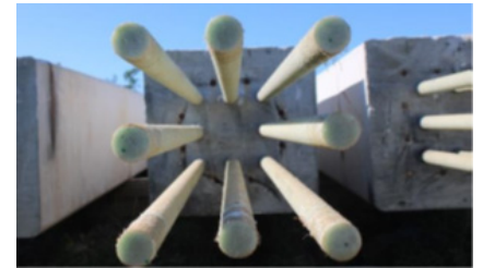
Research has been done to test the strength of a more cost effective material for dowels. Here, Glass Fiber-Reinforced Polymer dowels are being tested.
