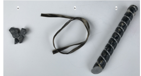
In a recent study, an FDOT research team evaluated basalt fiber reinforced polymers (BFRP) to be used in bridge infrastructure. Pictured l-r: basalt rock, basalt fiber, and BFRP.
