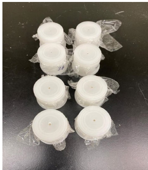
d) Sliced layers kept in sample cups ready for XRF measurements
