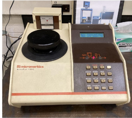
a) AccuPyc 1330 Pycnometer device
