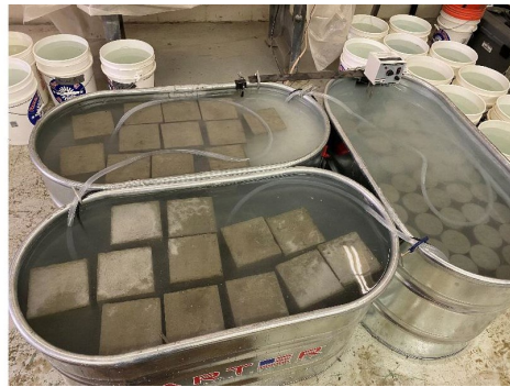
b) Curing tanks used to store the specimens
