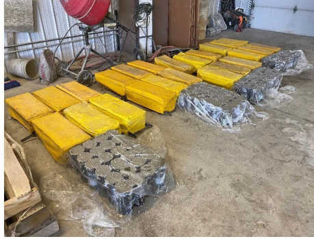
a) Beam and cylinder test specimens cast in the field
