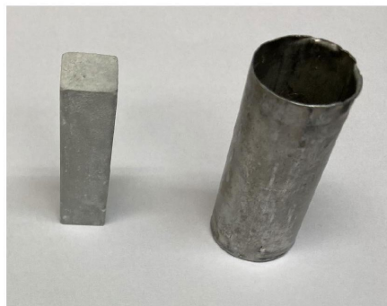
b) Chamber and a cement paste specimen
