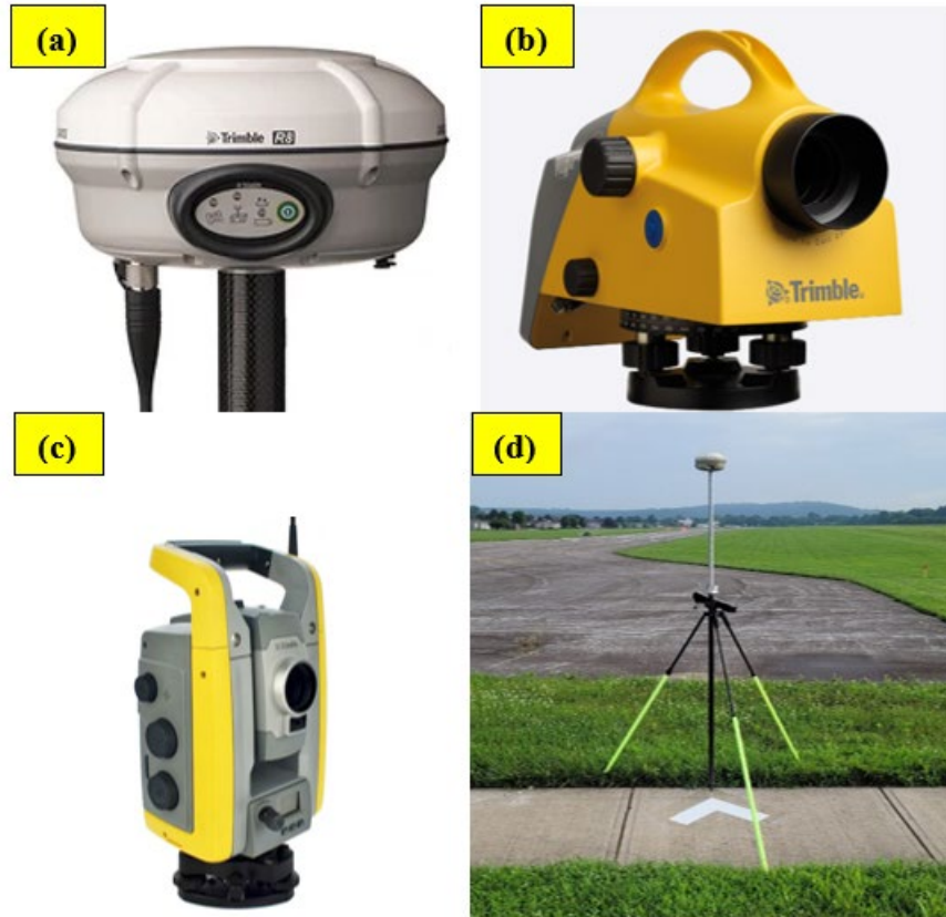
Figure 2. Survey Equipment: (a) Trimble R8 Model 3 GNSS Receiver, (b) Trimble S6 Robotic Total Station, (c) Trimble DiNi Digital Auto Level, and (d) Trimble Collapsible GPS Rover Rod with Tripod
