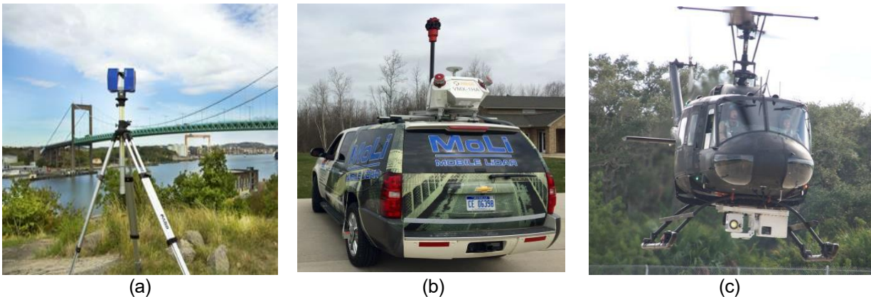
Figure 1: Example LiDAR platforms: (a) ground-based (courtesy of Faro 2015); (b) mobile (courtesy of SSI 2016); and (c) aerial (courtesy of JPL 2012).
