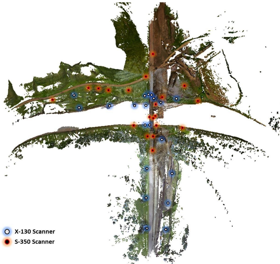
Figure 19. Scan setup locations for X-130 and S-350 laser scanners.
