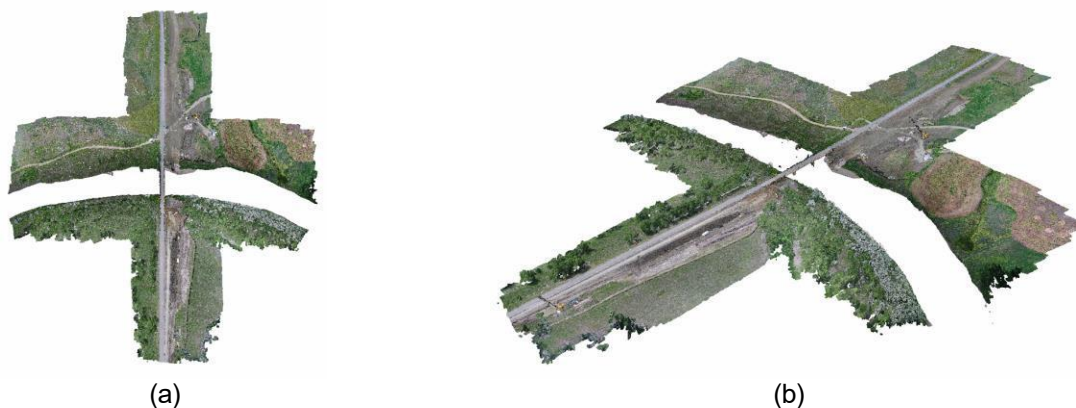
Figure 25. White River bridge SfM point cloud: (a) top view and (b) southeast isometric view.
