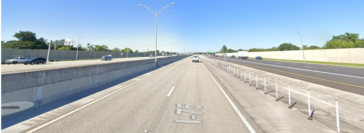
Figure 2.5: Concurrent Flow Express Lanes along I-75 in Florida (Source: Link )
