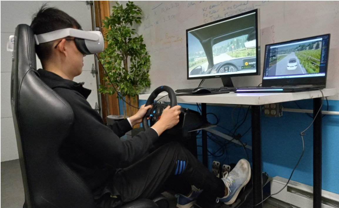
Fig. 12. Simulator demonstration: left monitor shows Carla server first person driver's seat view; right monitor shows the Carla client third person tracking view.
