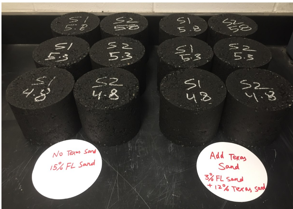
Figure 4-2. Granite SP-9.5 Specimens with and without Texas Sand (75 Gyration)
