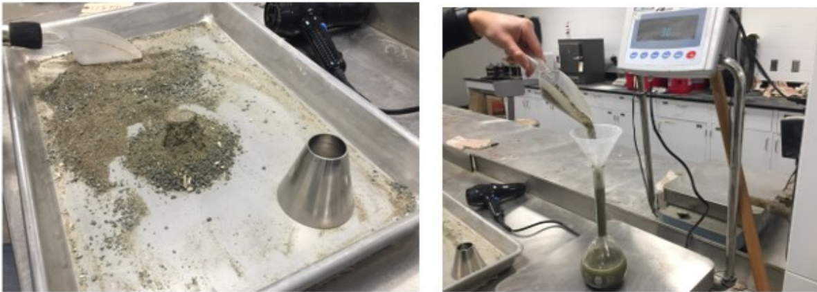
Figure 3-14. Fine Aggregate Specific Gravity Test
