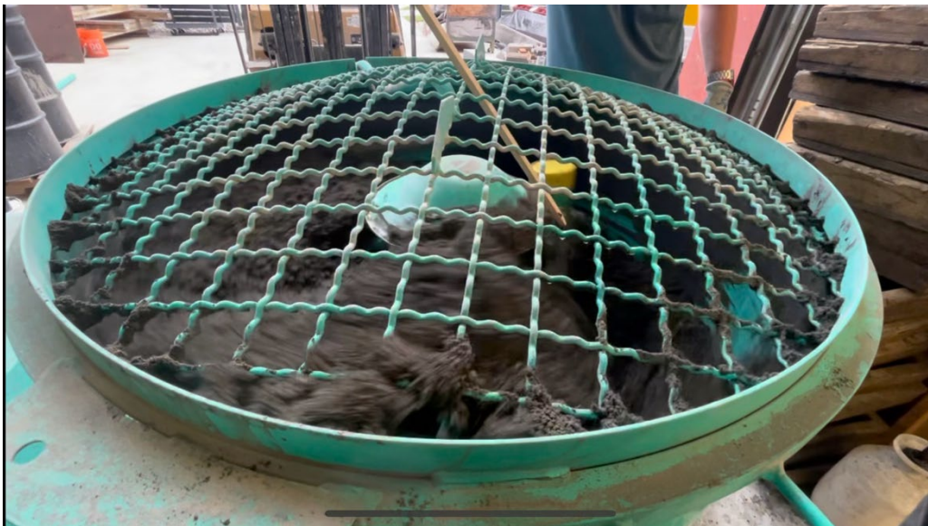
Figure 8: Mix constituents nearly overflowing during a 4.5-ft 3 batch
