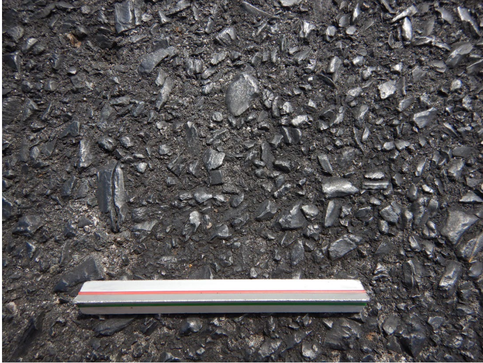
Figure EQY-18. P-632 Surface Texture on High Age Taxiway
