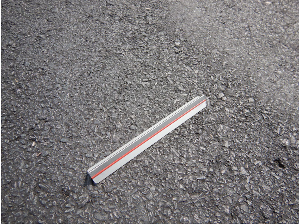
Figure EQY-10. Surface Texture of P-632 on Medium Age Taxiway
