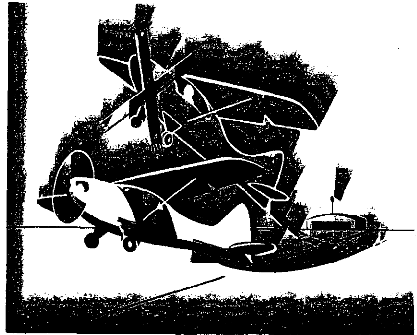
Figure 20. Climbing at a steep angle during a take-off is not only inefficient but also dangerous.
