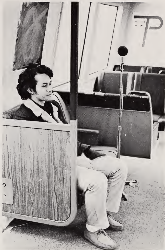
Noise levels are measured inside moving transit cars as part of UMTA's assessment studies.
