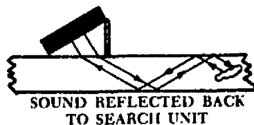
FIGURE 19. Reflection of ultrasound.
