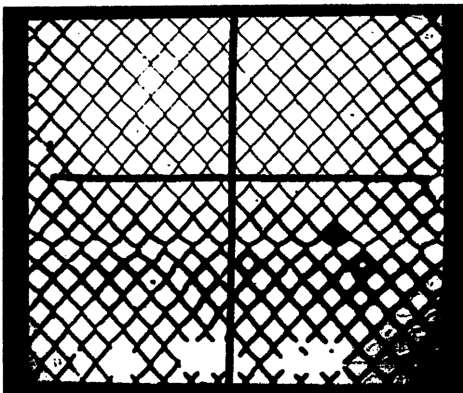
FIGURE 53. Ultrasonic recording of brazed honeycomb panel.
