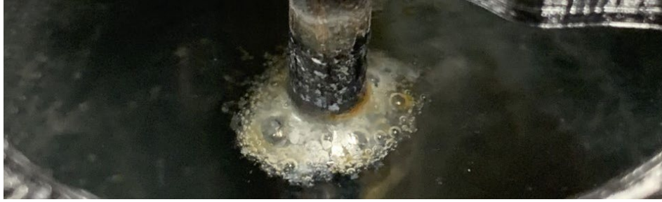
Figure 4-9. A photo of a galvanized steel duct filled with an aggressive water solution after one week of exposure showing hydrogen bubbles forming on the surface of the steel.
