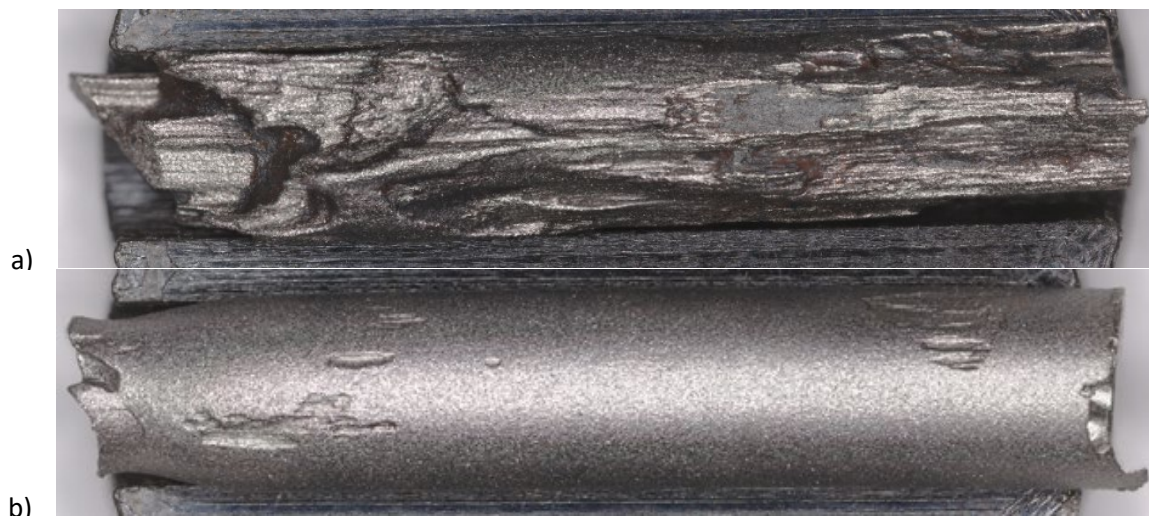
Figure 3-9. 3D surface images of corroded wire sections near the fracture location; (A) extensive corrosion with brittle fracture; (B) mild corrosion with ductile fracture.
