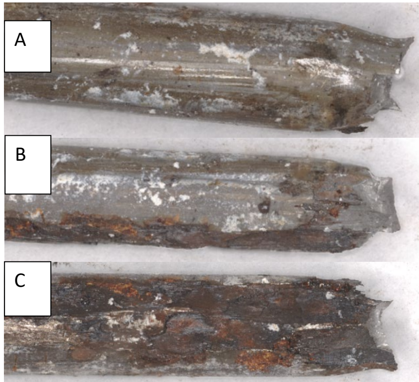
Figure 3-8. Different sides of the same wire showing: (A) inner surface of the wire without corrosion; (B) surface that contacts the neighboring wire with mild corrosion; (C) outer surface of the wire with moderate corrosion.
