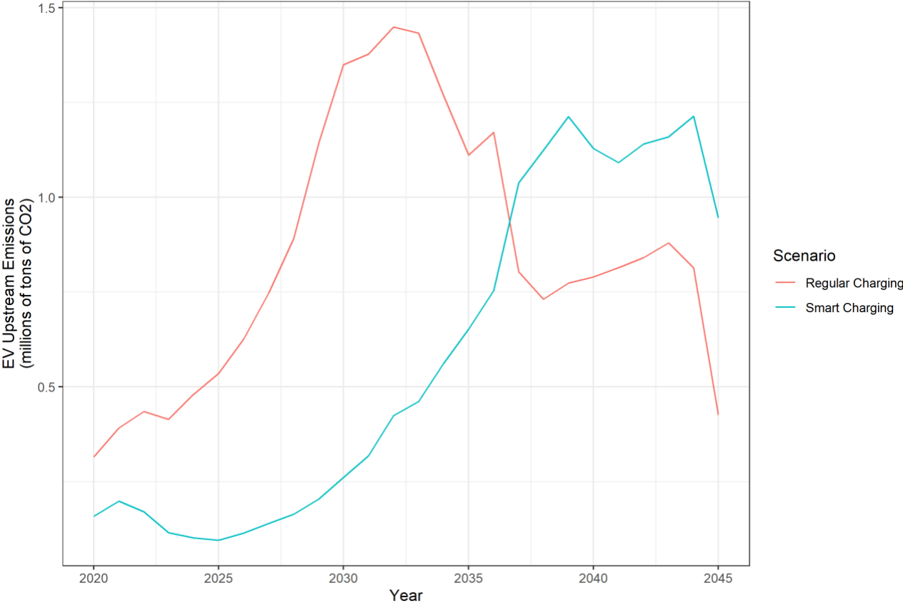
Figure 16. Total upstream annual emissions from the electricity grid for EV charging in two scenarios of charging (regular versus smart charging behavior).
