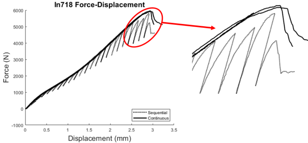
Figure 4.6: Softening and sharp load drop in In718 sequential test
