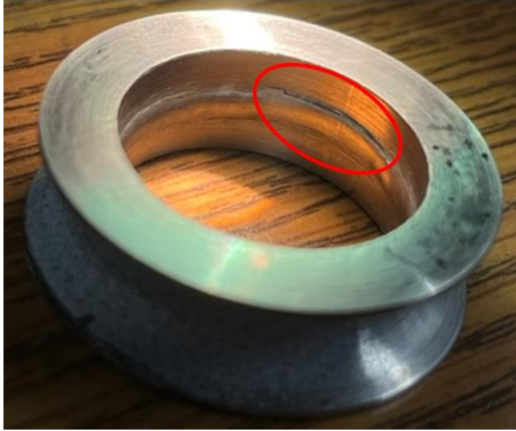
Figure 3.10: Fracture on inner ring surface on Ti64 specimen with 1 mm wall thickness
