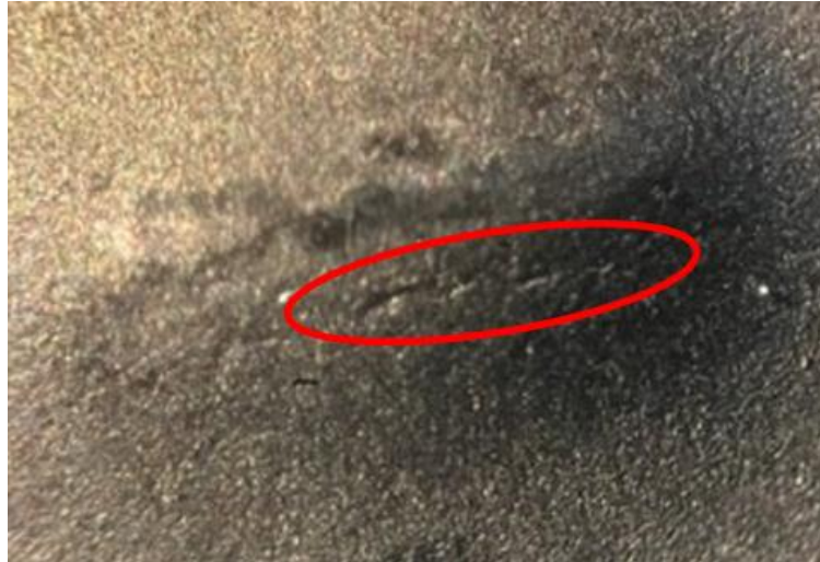
Figure 4.5: Fracture on In718 specimen where loading is stopped before load drop
