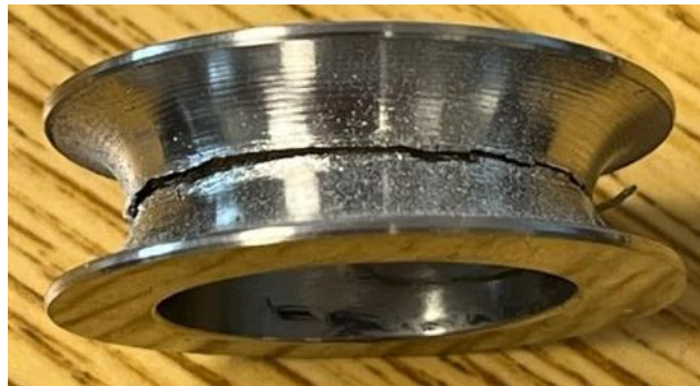
Figure 4.24: Normalized cumulative hit energy from a Ti64 test (top). The massive energy spike and load drop at the end is due to severe buckling and crack propagation (bottom). The crack propagates through the entire thickness of the specimen.
