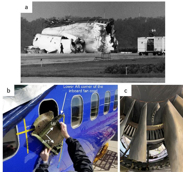
Figure 1.1: (a) Crash site of United Airlines Flight 232, (b) debris and site of detached window of Southwest Airlines Flight 1380, and (c) fractured fan blades on United Airlines Flight 328
