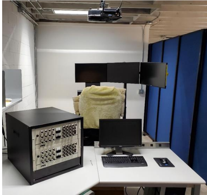
Figure B-3. Flight simulator operator station and control loader
